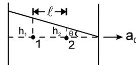
$$p_1 - p_2 = \rho a_0 l \quad \text{where } p_1 \text{ and } p_2 \text{ are pressures at point 1 \& 2. Then } h_1 - h_2 = \frac{l a_0}{g}$$
