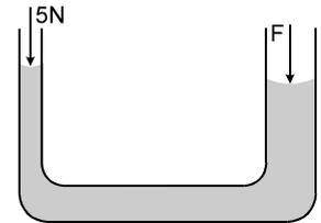
**Sol.** In equilibrium, the pressures at the two surfaces should be equal as they lie in the same horizontal level. If the atmospheric pressure is  $P$  and a force  $F$  is applied to maintain the equilibrium, the pressures are
