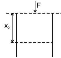
downward force =  $F + W = \text{Buoyant} = Ax_2 \rho g \dots (2)$
