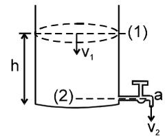
$$av_2 = a'v_3 \Rightarrow v_3 = \frac{av_2}{a'} \Rightarrow \frac{1}{2}\rho v_2^2 + \rho gh_0 = \frac{1}{2}\rho \left(\frac{av_2}{a'}\right)^2$$
