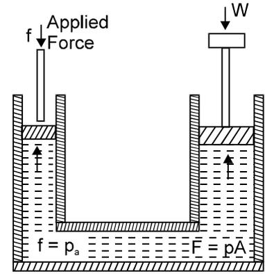
**Ex.1** The area of cross-section of the two arms of a hydraulic press are  $1 \text{ cm}^2$  and  $10 \text{ cm}^2$  respectively (figure). A force of  $5 \text{ N}$  is applied on the water in the thinner arm. What force should be applied on the water in the thicker arms so that the water may remain in equilibrium?
